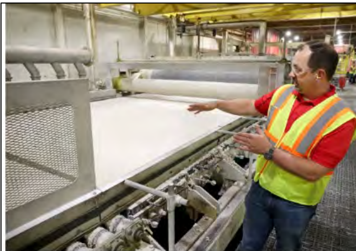
USG operations manager Matt Boyer talks about the process of the moist tile board being shaped before going into the dryer during a tour of the business in Cloquet on Wednesday morning, June 14. Jed Carlson / Superior Telegram
